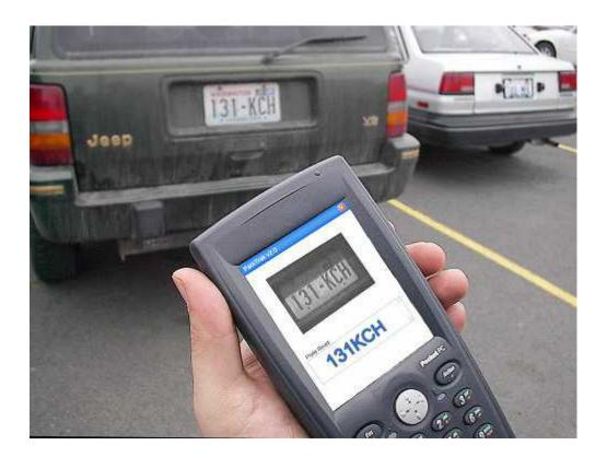
The portable unit can be used for license plate inventory, parking enforcement applications and parking data capture. It can also be combined with GPS system to provide additional location data.
